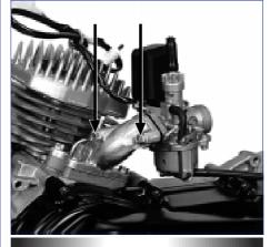
Removal of the reed valve and intake pipe
